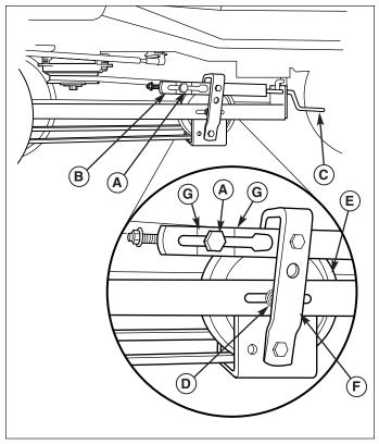
Figure 8. Adjusting Belt Tension
